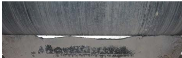
The mono-blade products on the market do not fit the belt
