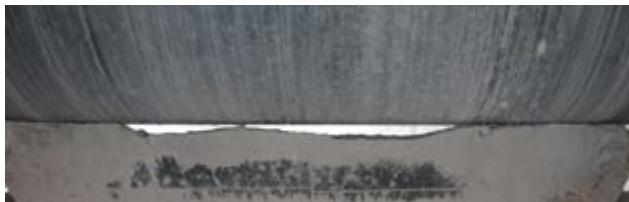
The Competitors' simple mono-blades cannot adapt to the belt
