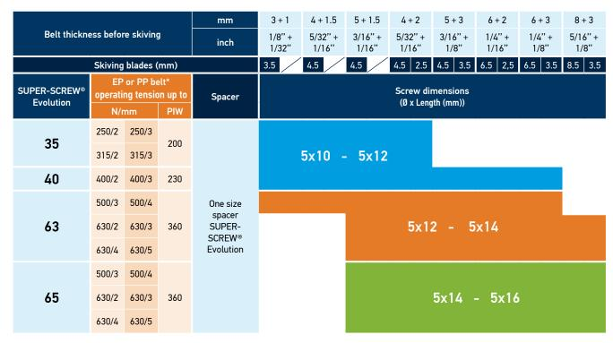
Template can be used with EP or PP (PN or NN) multiply belt
