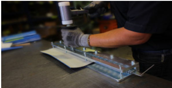
Self-Lock® installation tool
