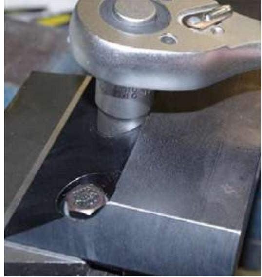
Once the blade arm assembly has been taken off, loosen the two M8 bolts that fix the blade to the support, with a 13mm key.
