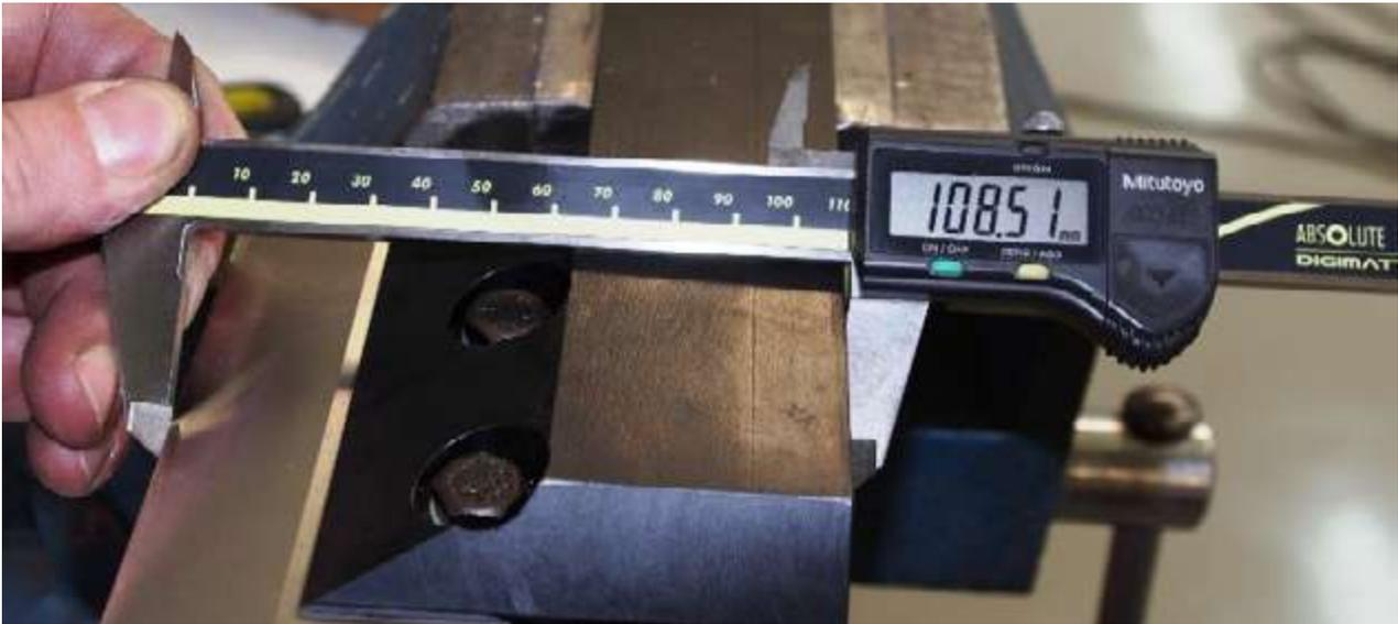
After changing the blade, reset the support to its original position by firmly tightening the two M8 Allen screws.
