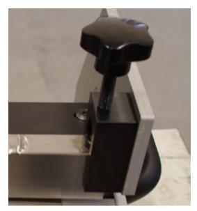
Once the belt is in position and complete fixed, push the down camp to liberate the step pin and move the head until end of stroke of GREEN side.
