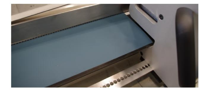
Once the head is in position to cut the second head of the belt, start to punch until end of stroke in YELLOW side.
