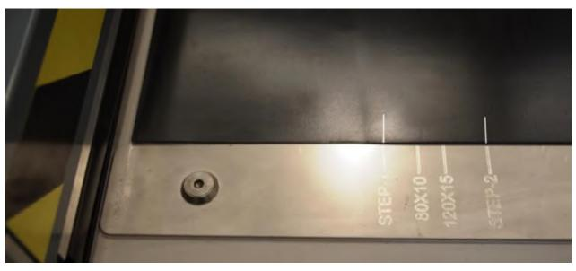
Then insert the material up to the first mark STEP-1.
