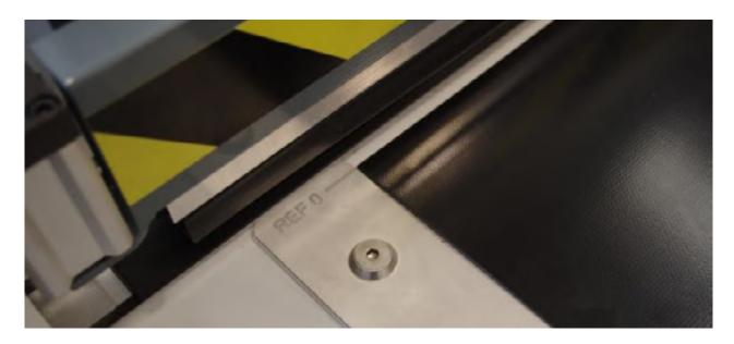
Then mark the measurement to input the relevant material with a pencil, according to the applicable die.
