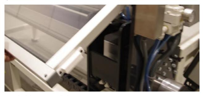
Loosen the 2 bolts using a 13mm Allen key.
