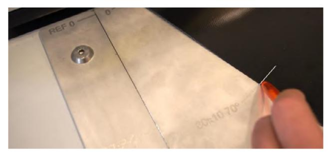
Then insert the belt until it aligns with the mark made at point «Ref 0»
