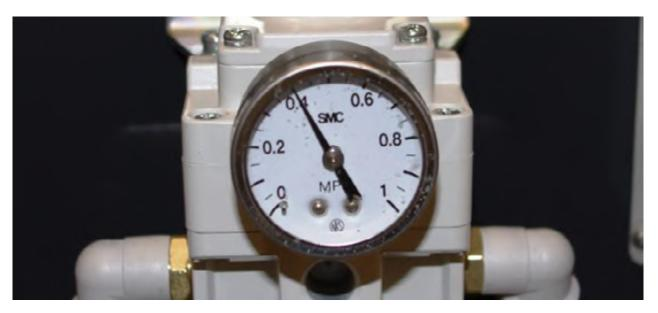
This adjusting device suffers a loss of air in order to keep the exact pressure constant.
