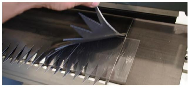
Once the plate has been placed inside, insert the material up to the second mark STEP-2.
