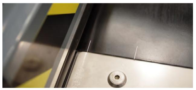
Lower the tread bar using the push button and press START. Once the first cut is completed, remove the excess material.
