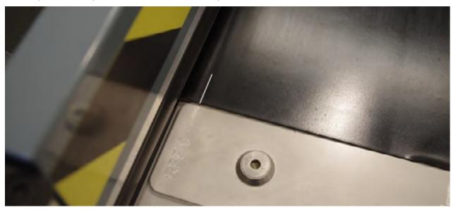
Reduce the cutting pressure to 2 bar, as the second cut will only cut the top fabric. Lower the tread bar and press START.
