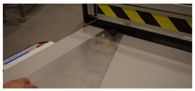
Place the belt that has already been cut in diagonal at  $70^{\circ}$  along with the supplementary guide to mark from «Ref 0» with the advance measurement of  $80 \times 10^{\circ}$ .
