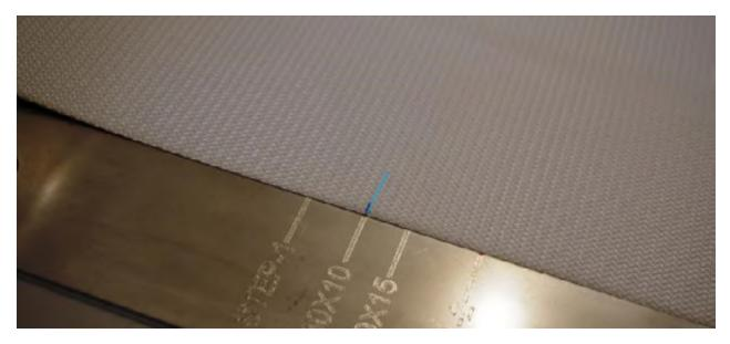
Next, feed in the belt under the holding bar until the mark aligns with «REF 0» and make sure it is fully in contact with the guide rail.
