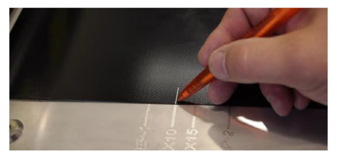
Place the belt under the tread bar until the measurement line matches up with «Ref 0» and make sure it is fully in contact with the guide rail.
